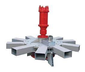
Power: 10Hp-50Hp Speed: 1450 rpm **Type SCLK** aerators / mixers are particularly suitable for deep tanks requiring high oxygen requirements; they are equipped with a submersible gearmotor and a slow-rotation impeller.
